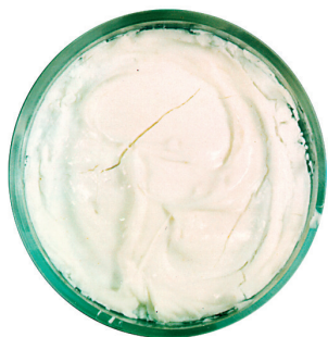
In oven at 232 °C (448 °F) for 40 hr: Krytox™—0% wt loss
